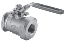
Seal Welded *Style BVSC Class 900 (2160 PSIG) R-PTFE Seats Sizes 1/4" - 2"
