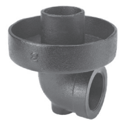
Cast Iron Drip Pan Elbow Style DPE Threaded or Flanged Sizes ¾" - 10" *6" & 8" elbows have 125# Flanges
