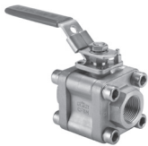
3-Piece Maintenance Design *Style BVM3 Class 800 1920 W.O.G. R-PTFE Seats Sizes 1/4" - 2 1/2"
